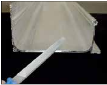
1) Before attempting to fit the adaptor, ensure that the inside edge of the Box Gutter is fully De-Burred.
